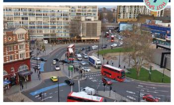
Multiple hazards entering roundabout as the bus must merge with other traffic across two lanes with vehicles turning left.
